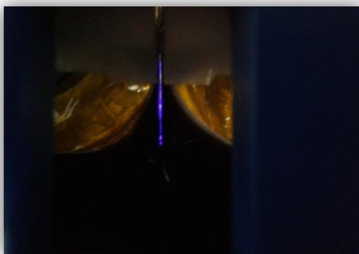
**Figure 1:** Atmospheric Pressure plasma formation between DBD rollers
