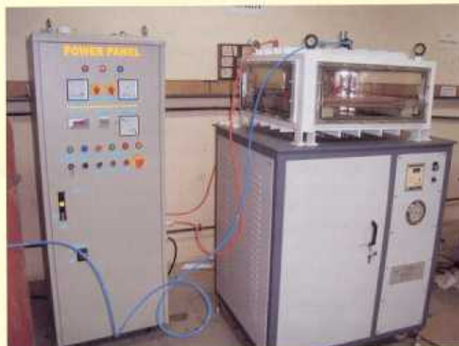
Fig. 1: Photograph of the atmospheric pressure plasma processing system, developed for WRA, Mumbai.
