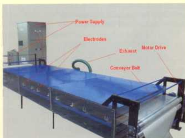
Fig. 2: Photograph of the industrial scale atmospheric pressure plasma processing system
