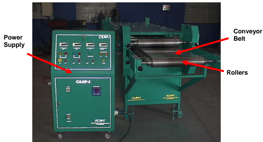
Figure 1 : Photograph of CAAP System
