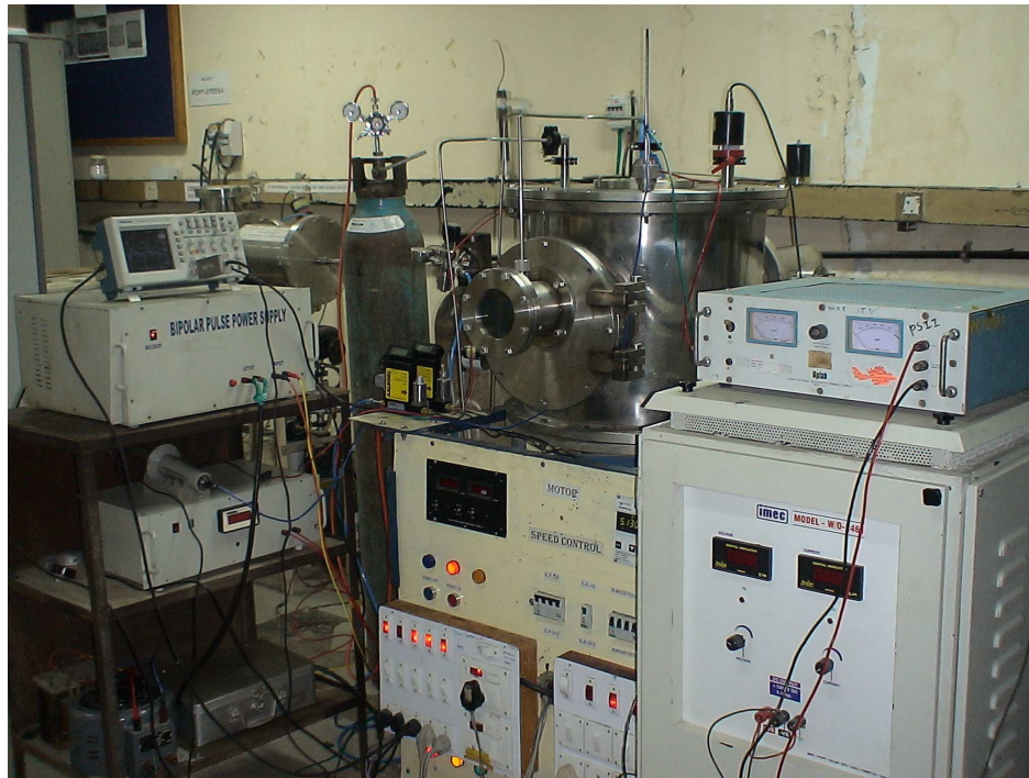
Fig.1 Photograph of the PVD based Titanium Nitride Coating system developed at FCIPT
