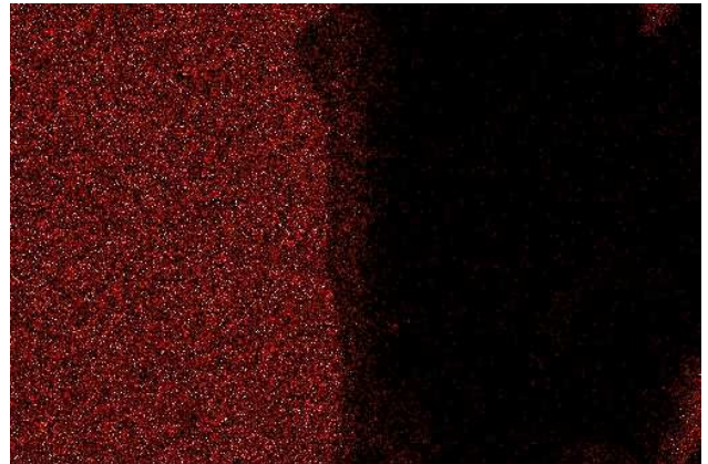
Fig-3d: EDX mapping of Cu at the interface
