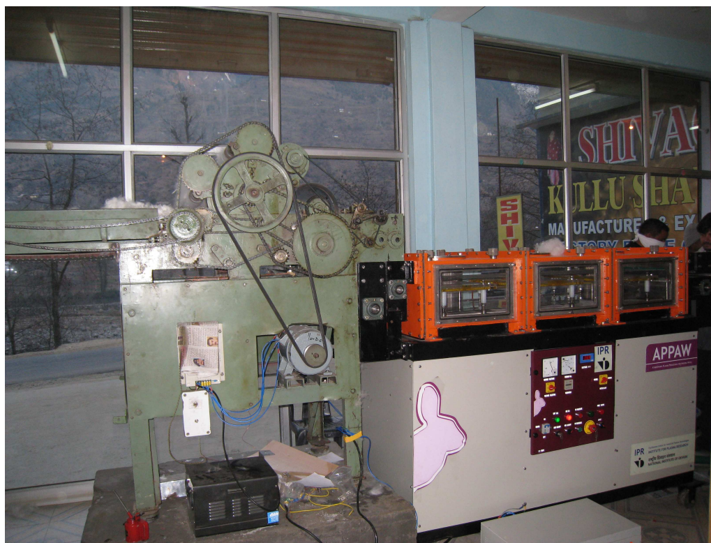
Fig. 1: Atmospheric Pressure Plasma System Installed at Kullu
