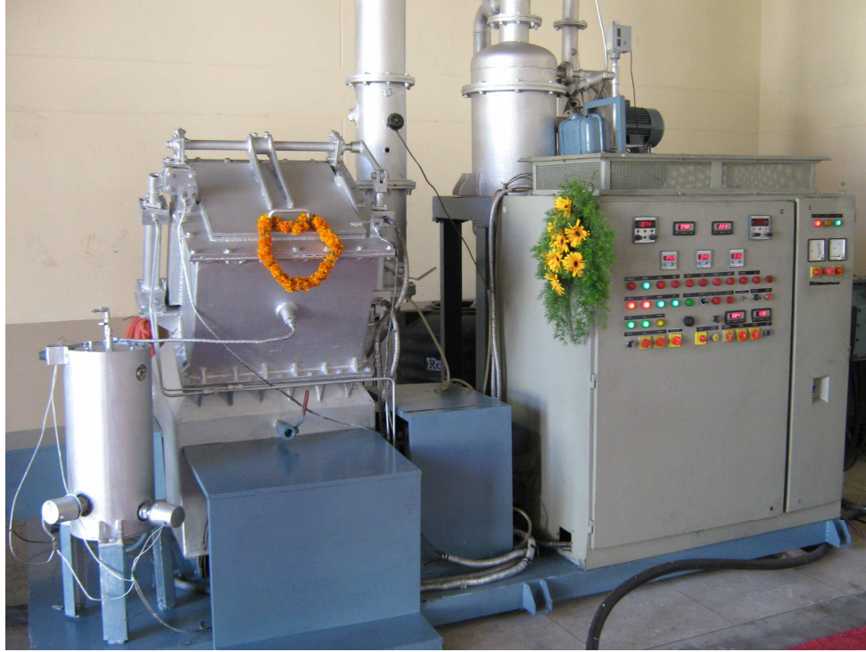
Fig. 1: Prototype plasma pyrolysis system for disposal of actual plastic and medical waste for demonstration and data collection in Gandhi hospital, Hyderabad
