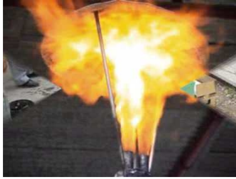
Fig.1 : Combustion flame of pyrolysis gas at the exhaust
