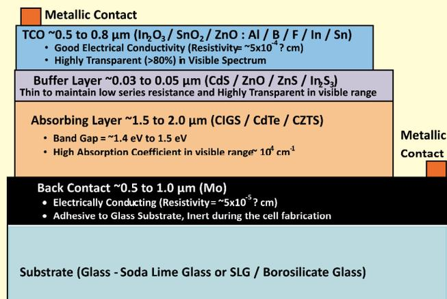
**Fig.1:** Typical Structure of Multilayer Thin Film Compound Solar Cell.
