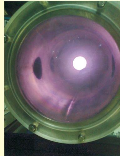
**Fig. 4:** Magnetron RF plasma
