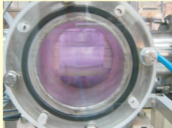
**Fig. 3:** Capacitively coupled RF PECVD Plasma
