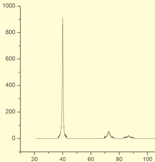
**Fig.3:** XRD results of Mo on glass thin Film
