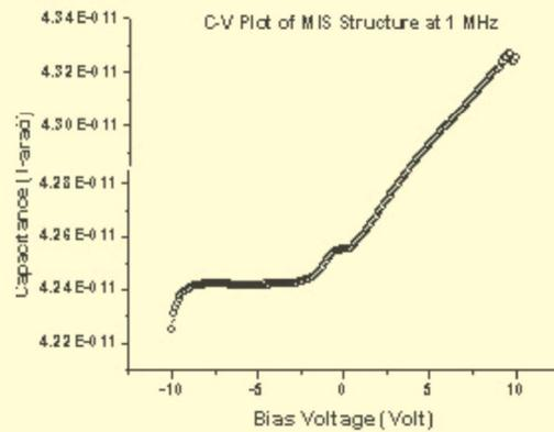
**Fig. 5(b): C-V Plot at 1 MHz**
