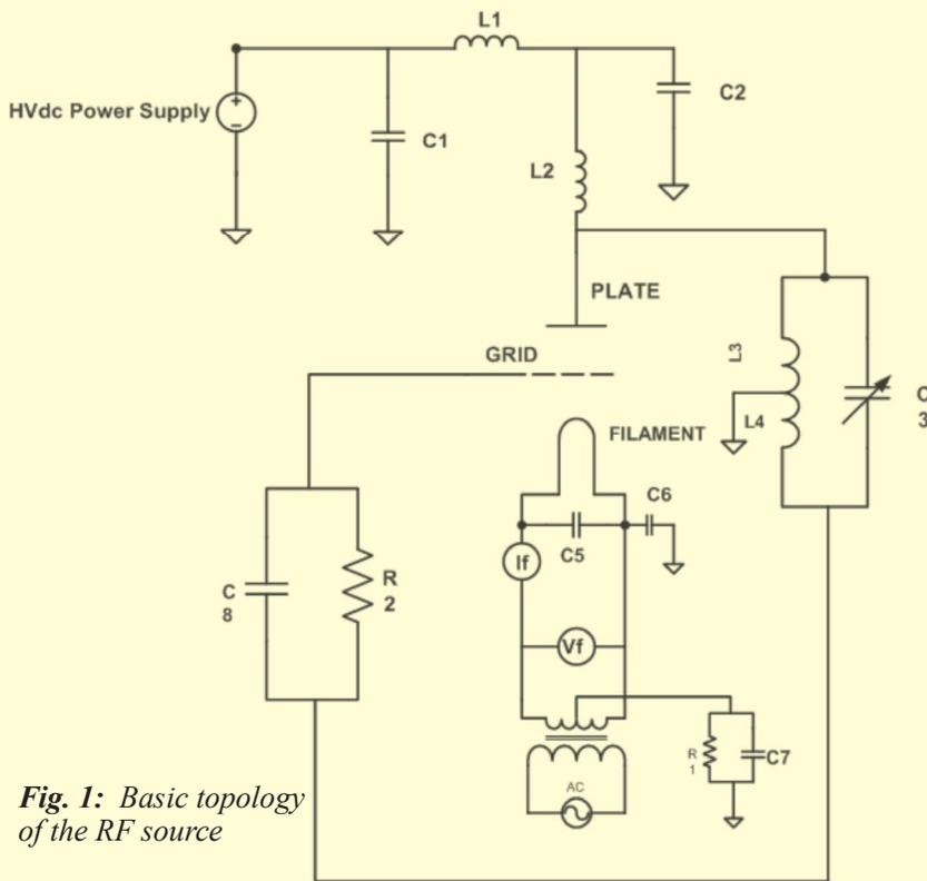
**Fig. 1:** Basic topology of the RF source
