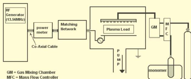
**Fig. 1:** Schematic of PECVD Deposition System
