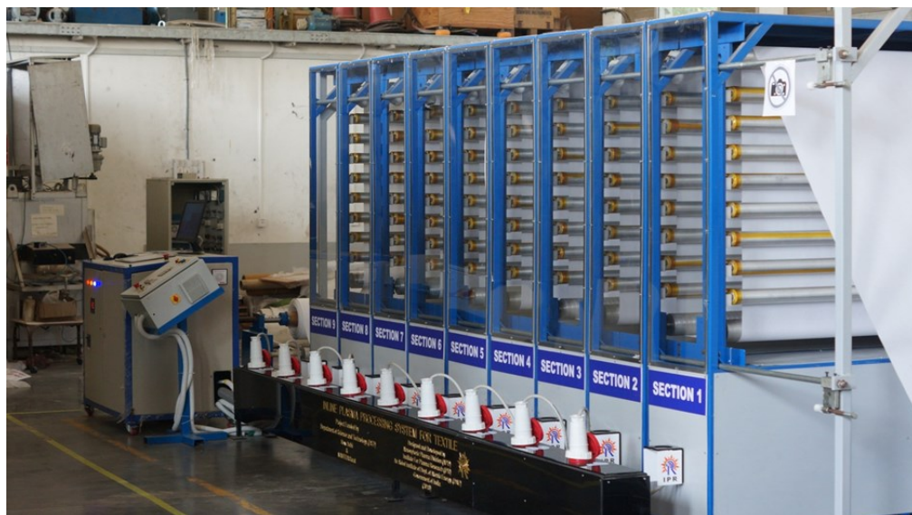
Figure 1. Plasma System for Inline Treatment of Textile
