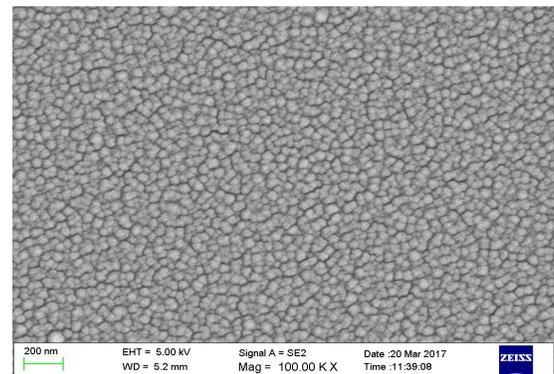
SEM image of Tantalum coating on silicon wafer
