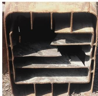
Fig. 2 : Eroded coal tip nozzle burner
