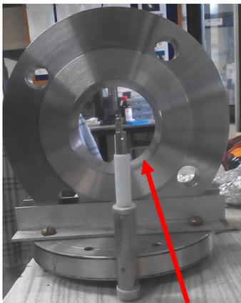
SS surface on which Tantalum coating is deposited
