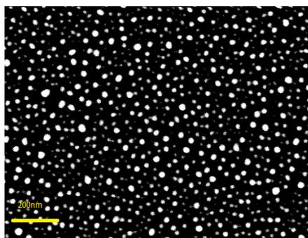
Left image is HRSEM image of Silver nanoparticles deposited on glass substrate.
