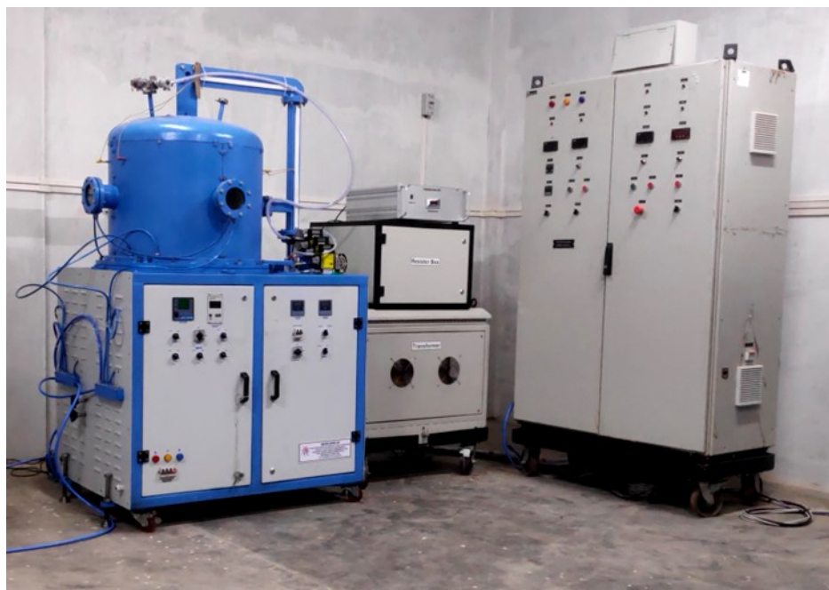
Plasma nitriding system installed at Dimapur Nagaland
