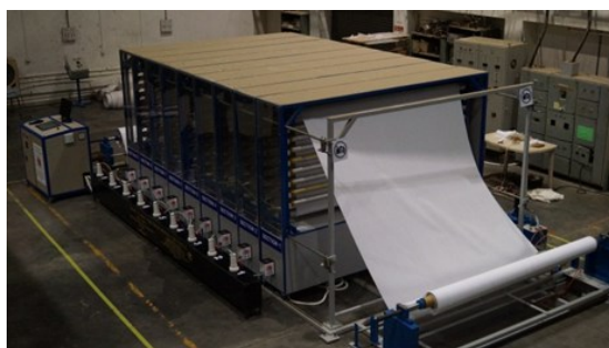
Plasma System for Inline Treatment of Textile installed at MANTRA, Surat
