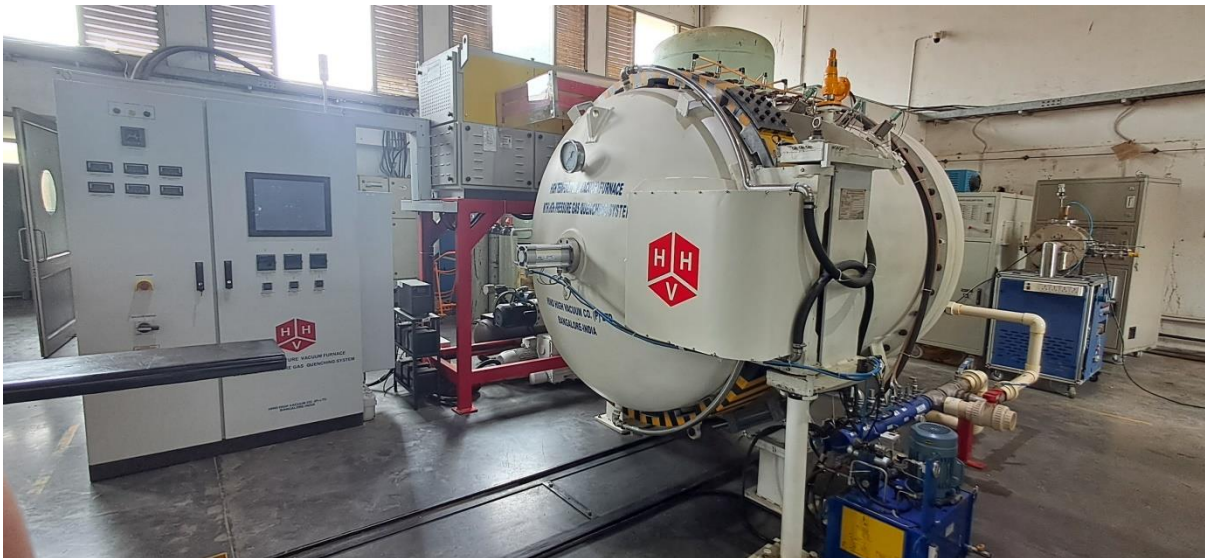
Figure 1: Plasma carburizing system installed at FCIPT
