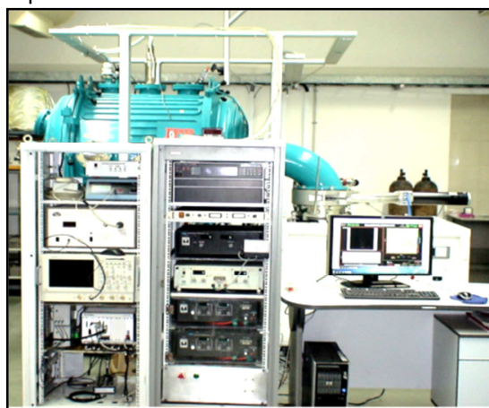
Fig 1: Experimental setup for testing arcing phenomenon
