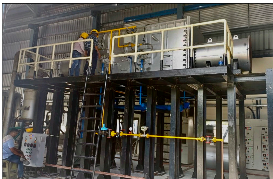
Secondary Chamber of 200 kg/h RAUDRA, installed at FCIPT, IPR
