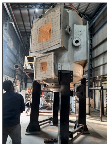
Primary Chamber during installation at FCIPT, IPR
