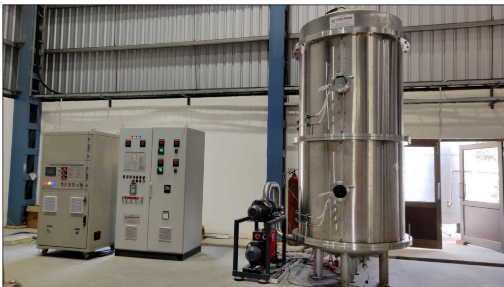
Figure 1: Plasma Nitriding system, recently installed at FCIPT, IPR
