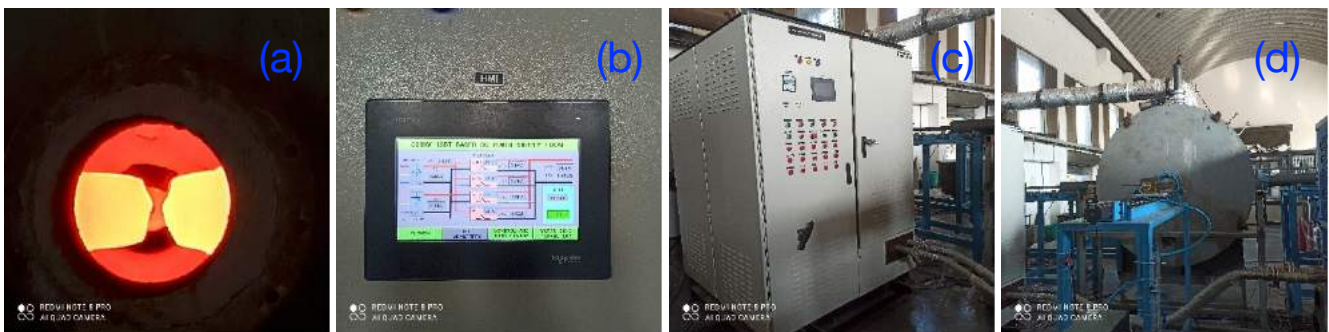
Figure 1: (a) Red hot electrode and chamber; (b) Control Panel; (c) Power supply unit; (d) Plasma torch test system comprising electrodes and chamber
